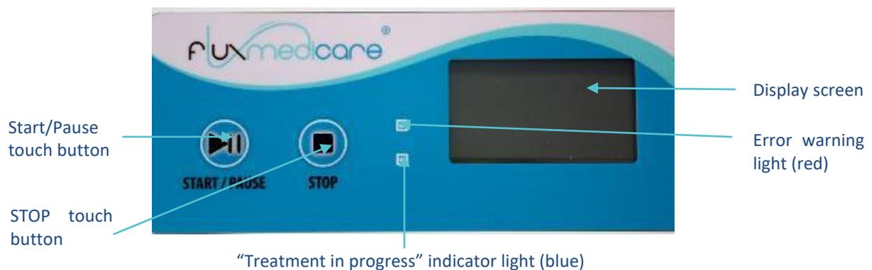
The front face of the light source (see Diagram 1) is made up of:
