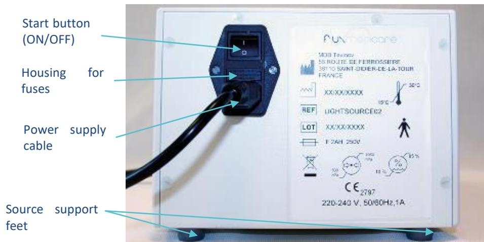
The rear face of the light source (see Diagram 2) is made up of:
