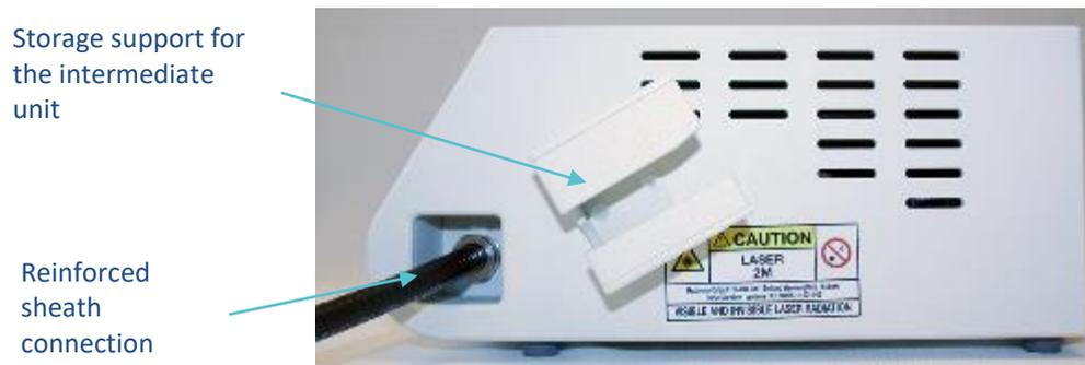
The right face of the light source (see Diagram 3) is made up of:
