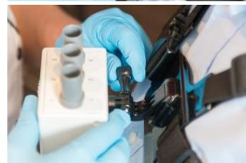
3. Connect the three connectors to the intermediate unit. These should be above the harness.
